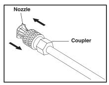
**STEP 3:** Insert nozzle into coupler. Release the coupler collar and push the nozzle until the collar clicks. Pull the nozzle to make sure it is seated properly.
