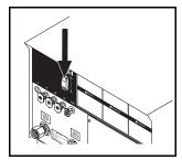
**STEP 2:** Turn off machine by pushing switch on front panel.
