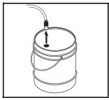
STEP 1: Remove detergent suction tube from soap container and insert into one gallon of fresh water. Use black soap nozzle with detergent injector. Pull trigger on spray gun and siphon water for one minute.
