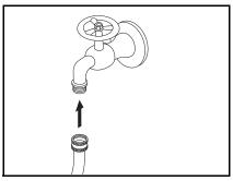
STEP 2: Connect garden hose to the cold water source. Before installing nozzle, turn on water supply and run machine, allowing water to flush through the system until clear.
