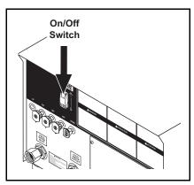
**STEP 3:** Turn machine on by pushing switch at front of machine.
