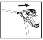
**STEP 2:** Apply safety latch to spray gun trigger. Secure black detergent nozzle into quick coupler. **NOTE:** Detergent cannot be applied using the Yellow nozzle.
