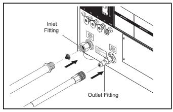
STEP 4: Connect the high pressure hose to the outlet discharge fitting. Push coupler collar forward until secure. Connect the garden hose to pump water inlet. Inspect inlets. CAUTION: Do not run the pump without water or pump damage will result.
