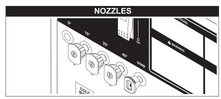
rīdæzfeve color-coded quick connect nozzles provide a wide array of spray widths from 0° to 40° and are easily accessible when placed in the convenient rubber nozzle holder, which is provided on the front of the machine.
