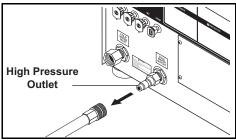
**STEP 6:** Disconnect the high pressure hose from high pressure outlet.
